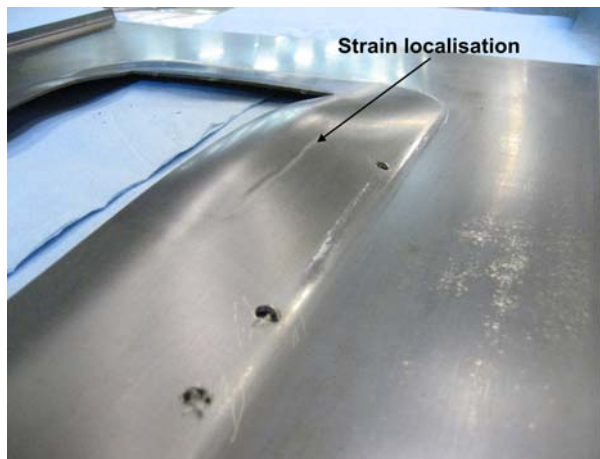
Figure 32. Photograph of the strain localisation which occurred in the hot forming of the Ti-6Al-4V sheet metal component (2).
