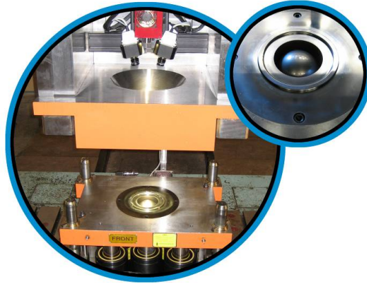
Figure 7. Illustration of the test setup for the forming limit tests (FLC).
