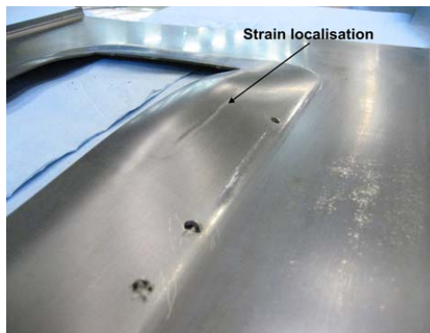
Figure 16. Photograph of the strain localisation which occurred in the hot forming procedure of the Ti-6AL-4V sheet metal component.
