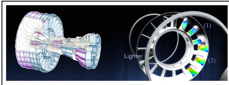
Figure 1. An example of a static load carrying aero engine structure containing sheet metal parts, ingots and forgings (nickel based alloys). FE analyses of shape deviation for sheet metal components.
